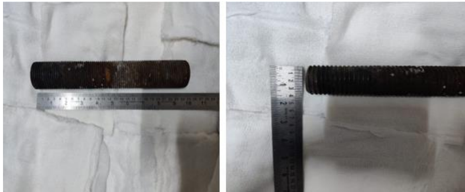
Figure 3: Retrieved iron rod which is 25 cm in length and 3.5 cm diameter
