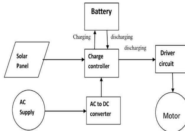
**Figure 1:** Block diagram of proposed design
