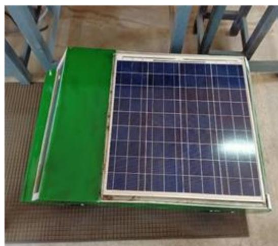
**Figure 2:** Solar Panel assembly of the Vehicle
