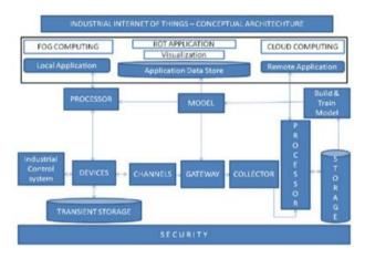
*Industrial Control System:* Industrial Control System is a general term used to define software and hardware integration to control critical infrastructure. They are generally developed using distributed control system (DCS), programmable logic control (PLC), supervisory control and data acquisition (SCADA) system, remote terminal units (RTU), control servers, human - machine interface (HMI), intelligent electronic device (IED) and many other industry - specific systems [1].
