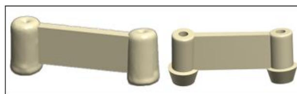
Figure 1. Designed of a virtual model of the suprastructures in software 3Shape Dental System ® after a) scanning of the abutments and b) scanning the scan bodies.
