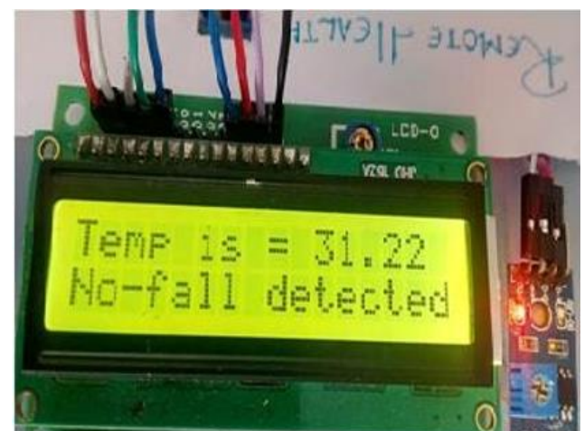
Figure 4.3: Status of fall detection and temperature
