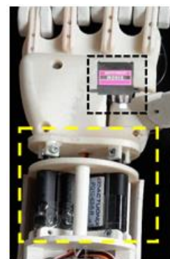
Figure 5: The black box illustrates the MG90S position to rotate thumb inward and outward. The yellow box shows all the string transferring from fingers to palm and then forearm with the servo wire and front facing linear actuator for wrist motion
