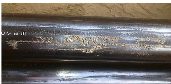
Figure 1: Power Cable Oversheath Fault
