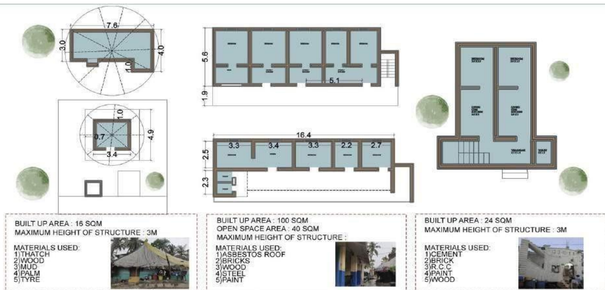
Figure 8: Showing the Planning of Fishermen Houses from 1980's to Present Model at Jalaripeta Fishermen Community
