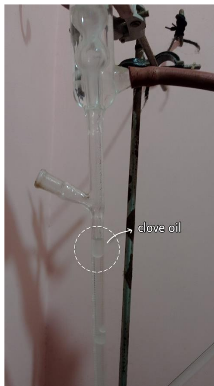
Image 5: Clove oil accumulation in collection tube
