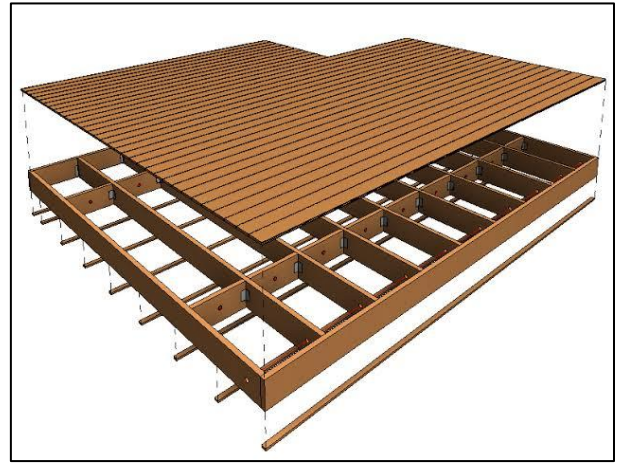
Figure 5: Framed Wooden Structure under wooden panelled flooring
