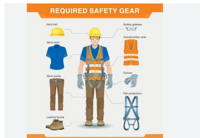
Figure 2: Safety Toot kit on Construction site for workers
