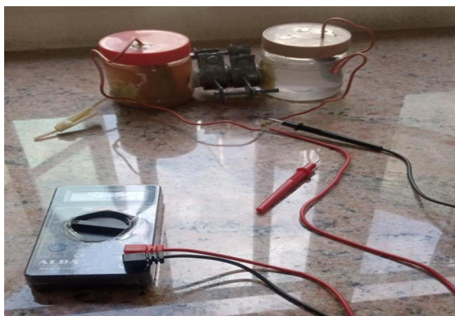
Figure 1: Two chamber MFC utilized during the MFC operation
