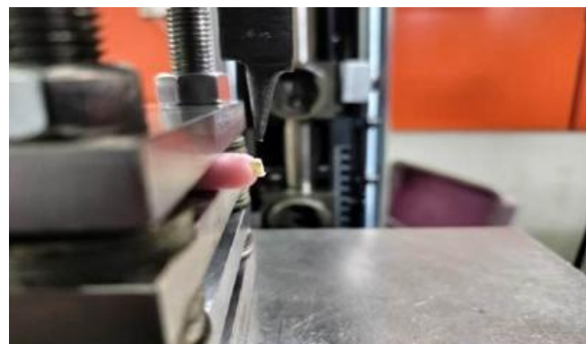
Figure 10: Sample fracture after maximum load resistance
