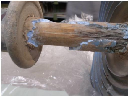
Figure 9: Traces of electrical erosion
