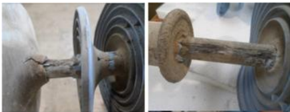
Figure 11: Silicon rubber FRP damages
