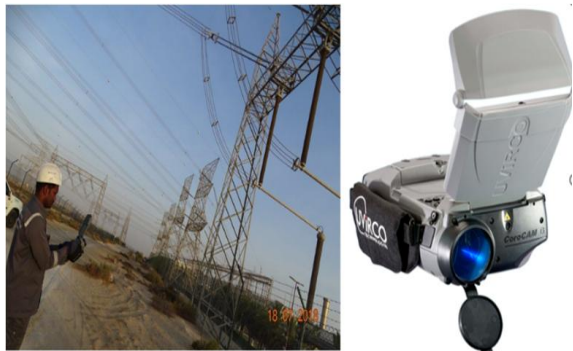
Figure 1: UV Site Inspection & UV Camera
