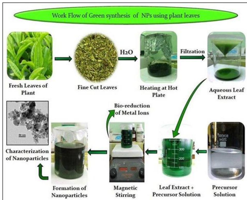
Figure 1: Work flow of green synthesis of nanoparticles using herbal plant leaves (Goutam et al. 2020) [14]
