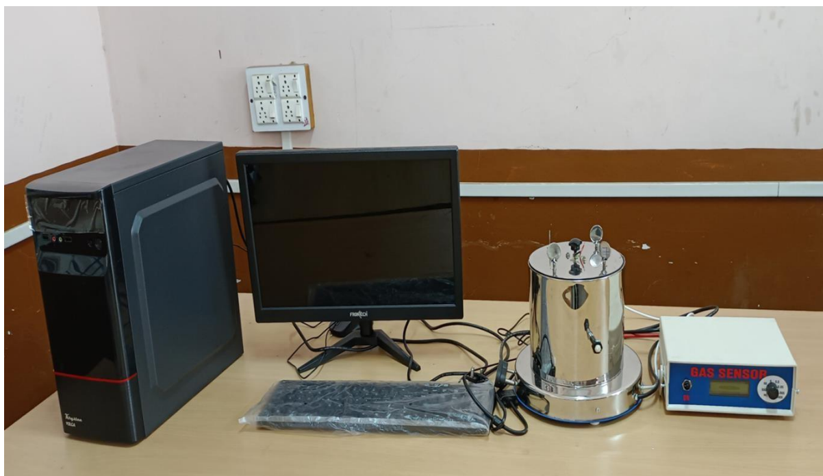
Figure 6: Shows experimental set up of gas sensor device.
