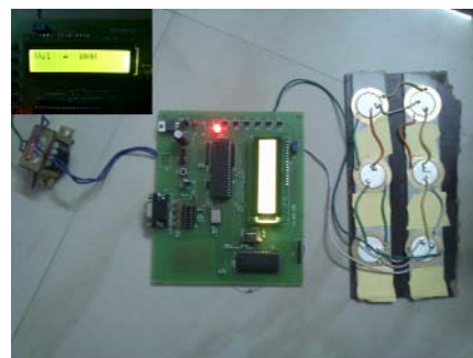
Figure 4: Voltage when no pressure applied
