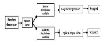
LDA seeks to reduce dimensionality while preserving as much of the class discriminatory information as possible. Assume we have a set of *D*-dimensional samples  $\{^{(1)}, x^{(2)}, \dots, x^{(N)}\}$ , *N*1 of which belong to class  $\omega$ 1, and *N*2 to class  $\omega$ 2. We seek to obtain a scalar *y* by projecting the samples *x* onto a line  $y = w^T x$
