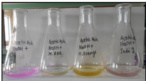
Figure 11: Titration of weak acid (Acetic acid) with strong base (Sodium Hydroxide) using Synthetic indicator (Phenolphthalein, Methyl red, Methyl orange, Natural indicator like Indicator-1, and Indicator -2)
