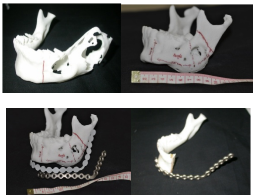
Figure 3: Fabricated Mandible model by SLS & Preoperative Study
