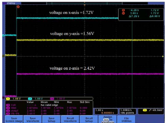
Figure 4: Accelerometer output voltages on three axes in static acceleration mode
