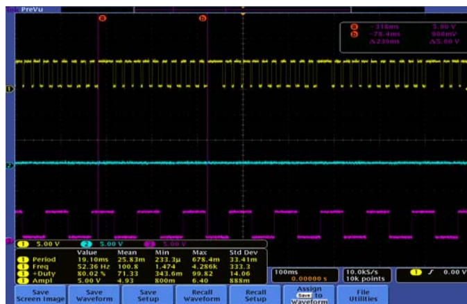
Figure 8: Response of proximity sensor on detection of a tooth of an encoder disc
