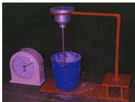
Figure 2: Measurement viscosity of investment slurry.
