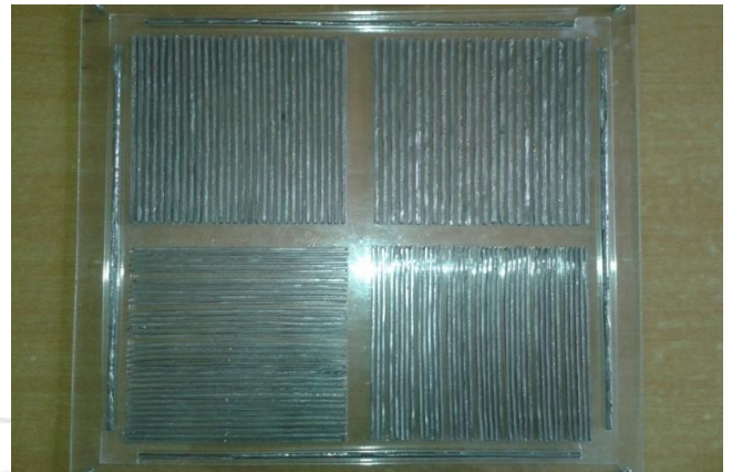
Figure 1: shows the frontal part of the phantom made of Perspex (42×42×10 cm) that simulates the four quadrant bars phantom each one was 20×20 cm
