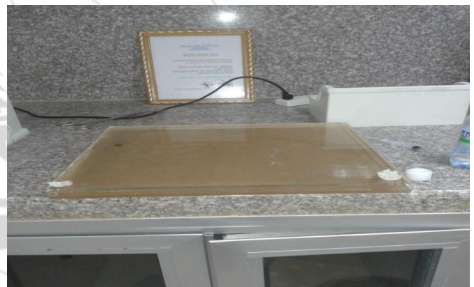
Figure 2: shows the back part simulates the liquid flood phantom made of Perspex (42×42×1 cm) and has orifice 0.5 cm to be fill with a liquid radioactive material
