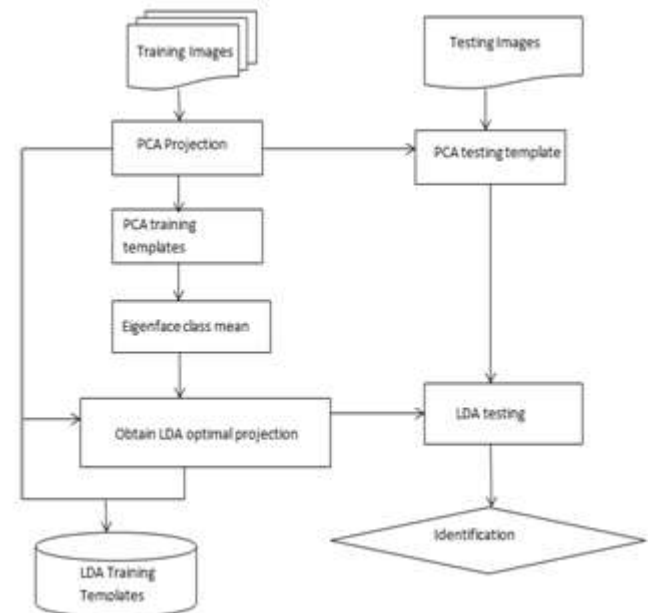
Figure 3: Simple flowchart of PCA algorithm
