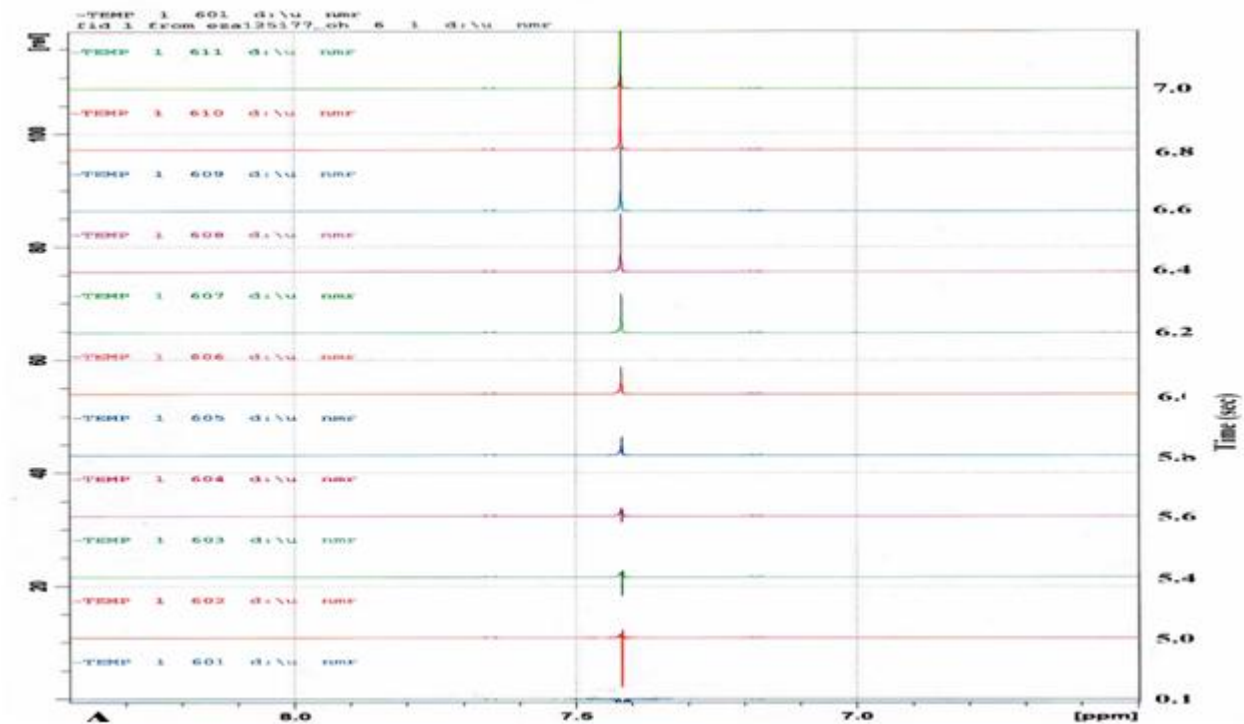
Figure 4: Schematic presentation of a typical evolution of line intensities in ^1\text{H} NMR spectra, collected by inversion recovery experiments at different values of \tau (at 400 MHz in DMSO, at 26°C) of bismaleimide BMI1.
