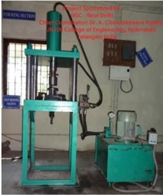
Figure 2: Deep drawing machine (hydraulic type).
