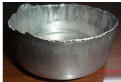
Figure 24: The successful deep drawn cup
