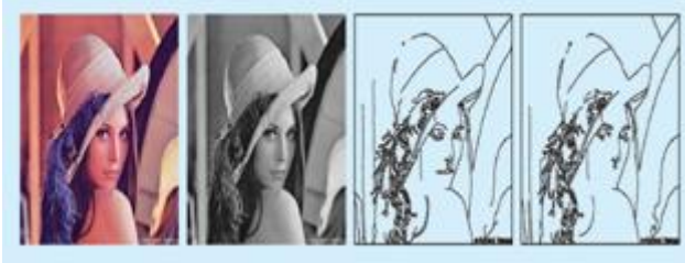
Figure 3: Results of edge detection applied to the color image Lena. (a) Original color image. (b) Gray-level representation. (c) Results for a color variant of the Canny operator. (d) Results of the gray-level algorithm of the Canny operator
