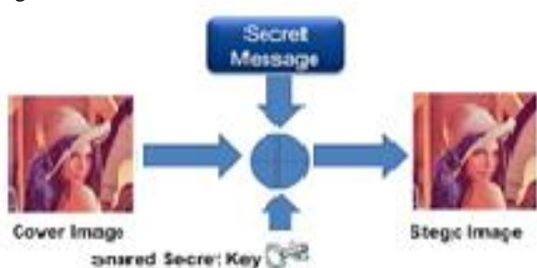
Figure 4: Basic Steganographic System
