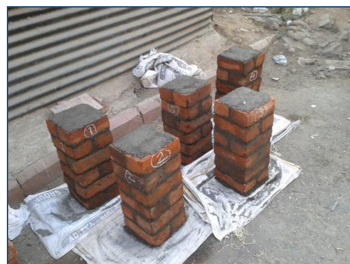
Figure 3: Brick Masonry Prisms
