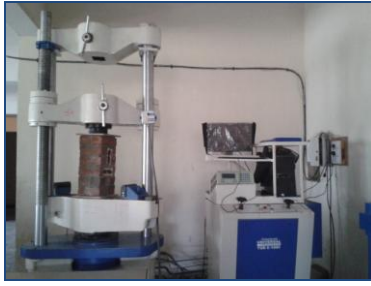
Figure 4: Testing of Brick Masonry Prism
