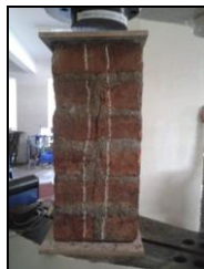
Figure 5: Vertical Splitting Cracks
