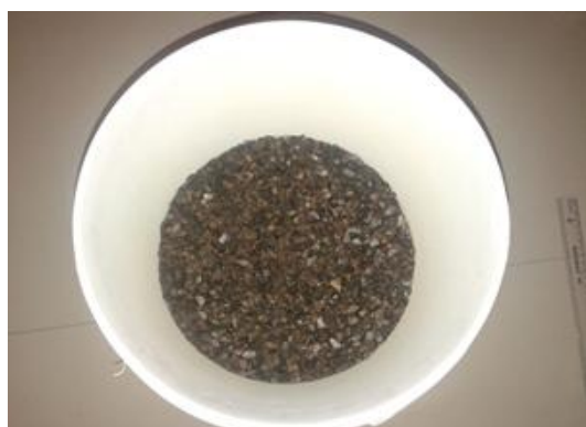
Figure 2: 2-3 cm size of gravel used in formation of vermifilter bed
