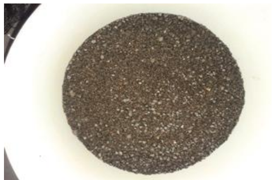
Figure 3: 1-2cm size of gravel used in formation of vermifilter bed
