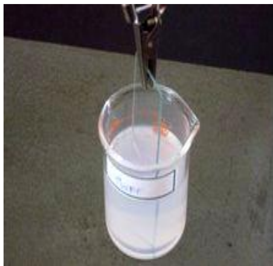
Figure 1: Chemical Bath Setup of a Cas thin film
