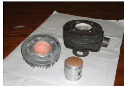
Plate 1 Photographic view of copper coated piston, liner and copper coated cylinder head of CCE
