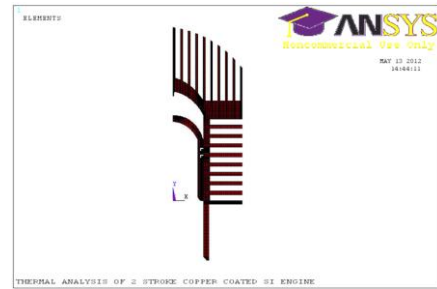
Figure 2 Mesh employed in the thermal analysis for CCE
