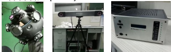
(a)Laser scanners (b) sensor (c) controller Figure 1: The reverse reconstruction process of UAV impeller
