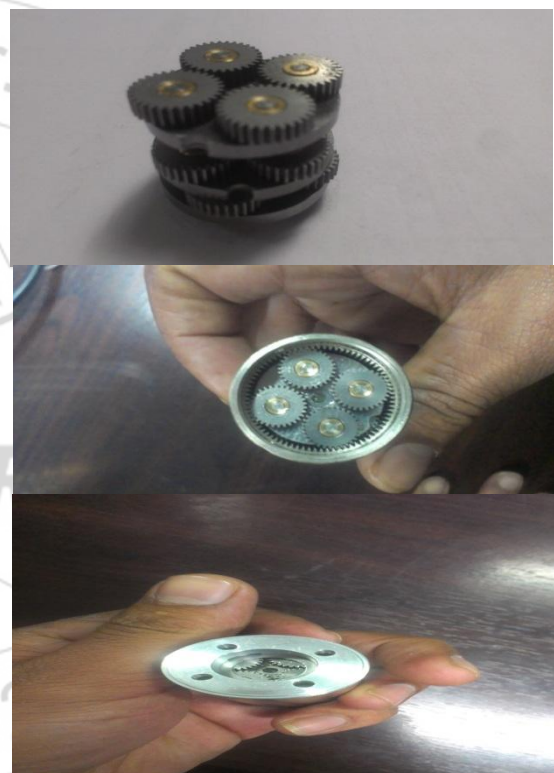
Figure 1: planetary Gearbox Internal view.
