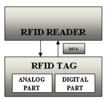
Figure 1: A simplified RFID system.
