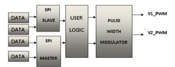
Figure 2: RFID- tag baseband architecture
