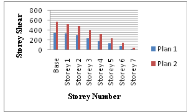
Figure 15: Storey Shear of G+6 Buildings (kN)
