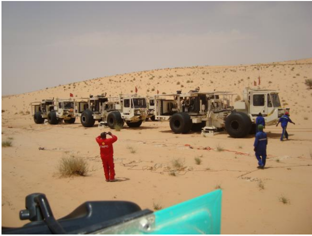
Figure 2: Vibrators in Source Array, with the Base-plate dropped to impact vibration waves into the ground.
