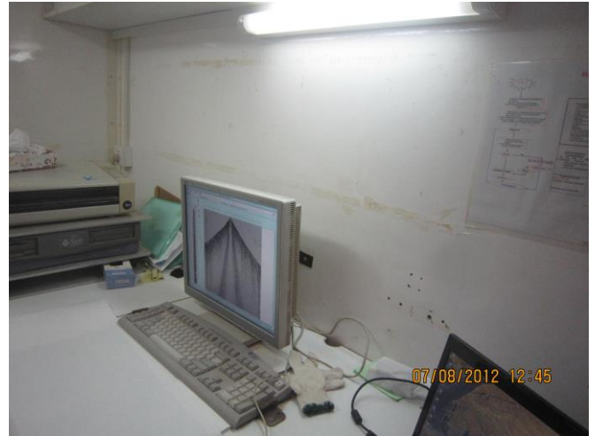
Figure 4: Inside the Recording Truck, Seismic data as the sweeps were to record, showing signal frequencies 30Hz to 60Hz with good amplitudes.
