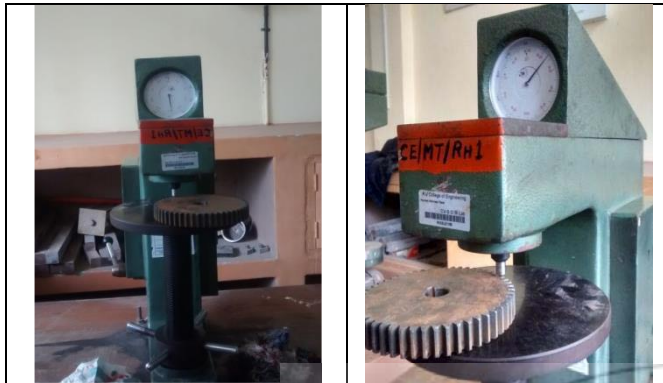
Figure 4.11: Hardness testing of gear using Rockwell hardness tester
