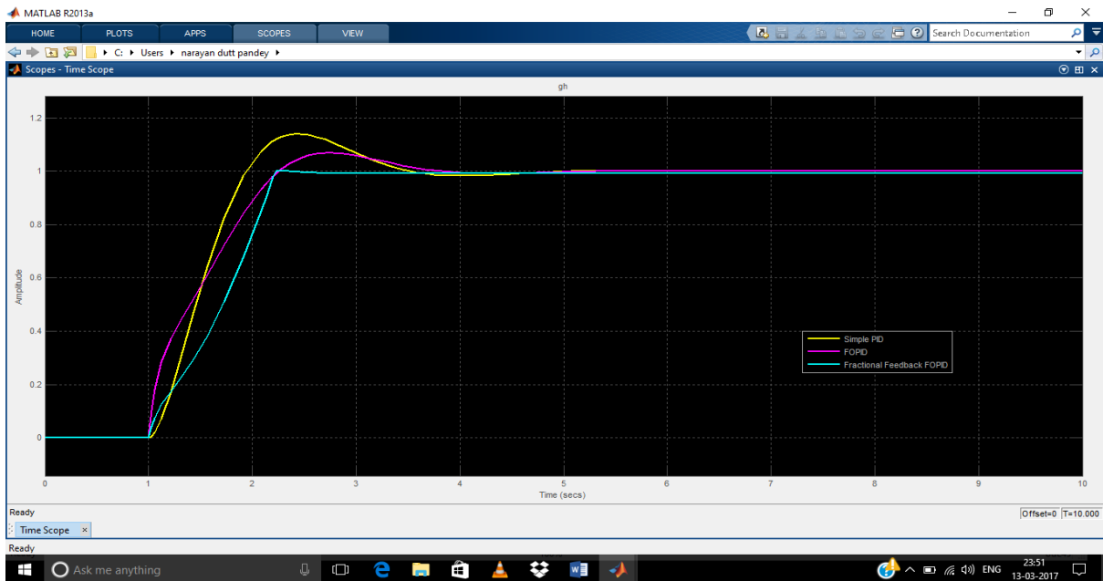
Figure 13: Comparison of Performance Parameters of PID, FOPID and Fractional Feedback FOPID Controller
