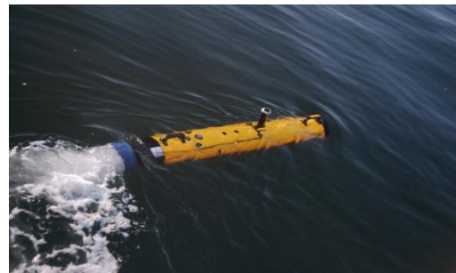
Figure 5: AUV to detect mine like objects
