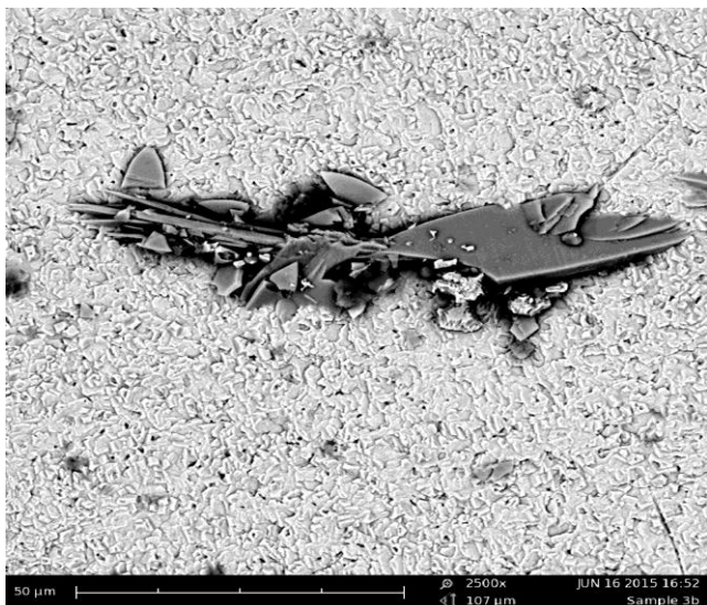
Figure 1(b): Annealed Cuprous Oxide layer produced by Immersion techniques at pH 5.5
