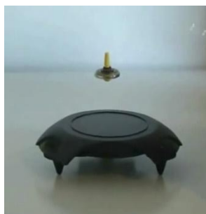
Figure 1: Magnetic levitation of a magnetic material
