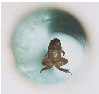
Figure 4: A picture of frog levitating inside a 32mm diameter vertical bore providing 16 Teslas of magnetic field
