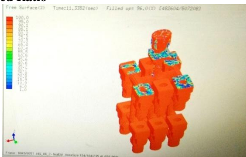
Figure 17: Filling ratio of twelve cavity gating system
