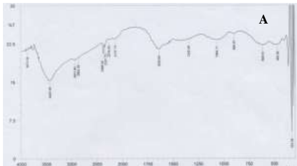
Figure 1: FTIR test results of bacterial cellulose produced by Gluconacetobacter xylinus at (A) 0 rpm (B) 50 rpm
