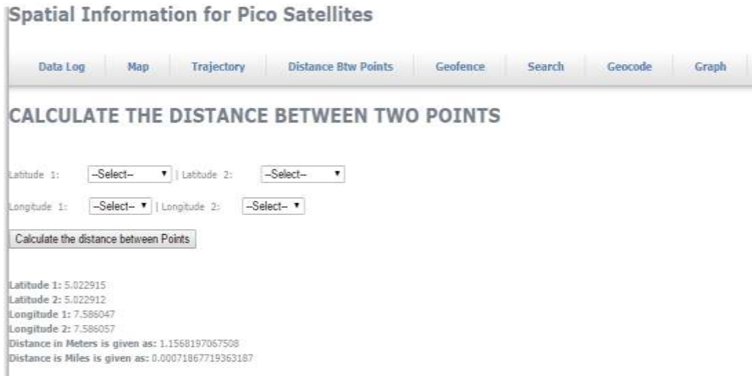
Figure 4.7: Screenshot showing the result of calculation of distance that spans amid two points
