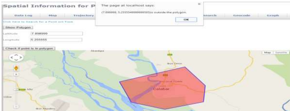
Figure 4.8: Screenshot showing how to ascertain the point that exists in the geo-fenced region
