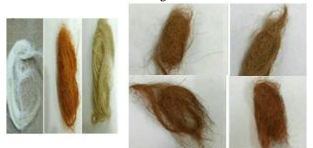
Figure 4.2: Coloring using henna and nickel when nickel concentration is stable and henna concentration changes.
