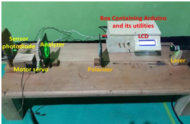
Figure 3: Hardware of light polarization tool based on Arduino
