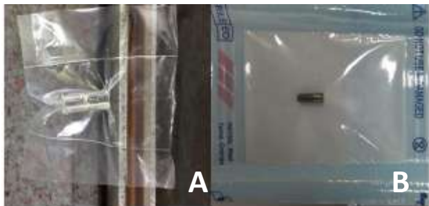
Figure 1: A: Screw stored in vacuum package, B: Screw stored in air
