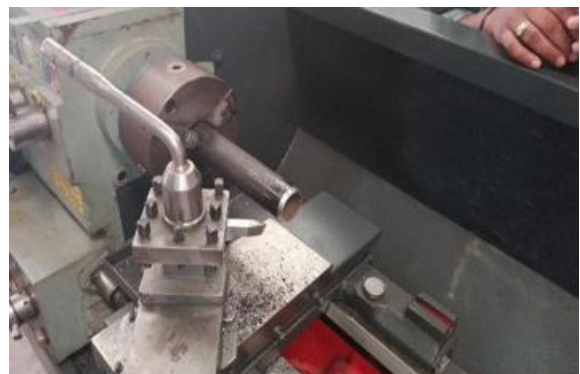
Figure 4: Grooving of Pipes
