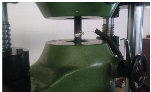
Figure 10: Pipe placed between jaws of UTM
