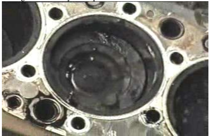
Carbon deposits on the piston bottom – the result of incorrect combustion
