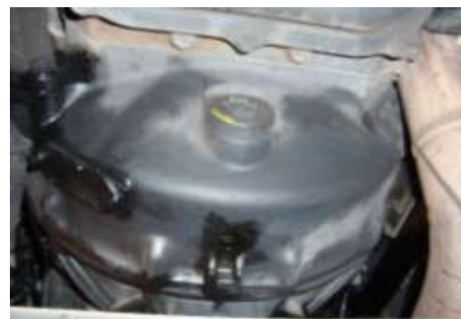
View of the front part of a gearbox housing (clutch – engine flywheel) that is contaminated with oil – oil leaking from an engine through a spring-energised seal.
