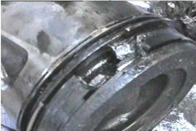
Detailed view of 2 nd cylinder piston after partial cleaning of carbon deposits
