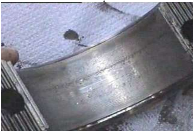
View of the 2 nd cylinder connecting rod bearing (bearing bushing of a connecting rod) – 2 nd part of a bearing (clamp)
