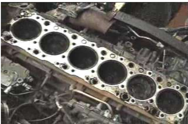
View of the engine block, cylinders and pistons after the disassembly of a cylinder head
